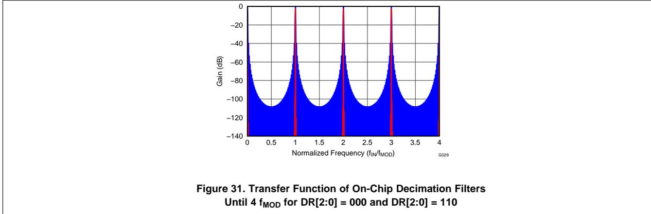
Figure 31. Transfer Function of On-Chip Decimation Filters Until  $4 f_{MOD}$  for  $DR[2:0] = 000$  and  $DR[2:0] = 110$
