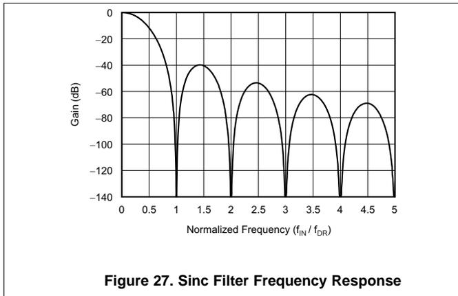
Figure 27. Sinc Filter Frequency Response
