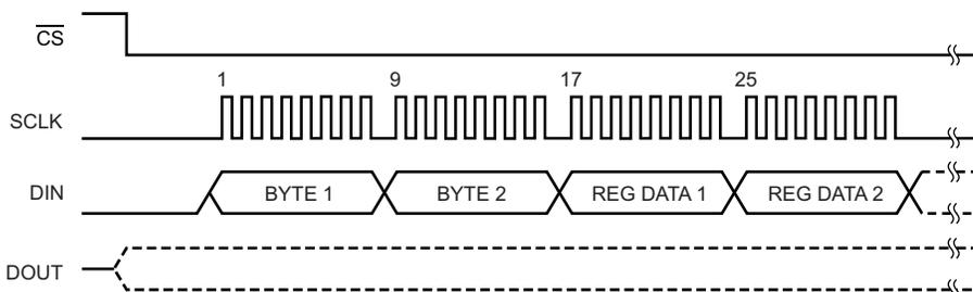
Figure 49. WREG Command Example: Write Two Registers Starting from 00h (ID Register)
