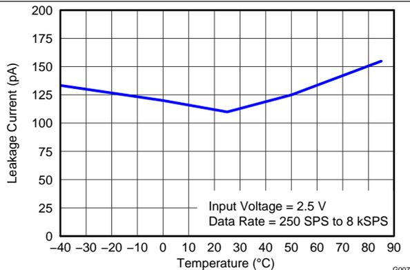
**Figure 7. Leakage Current vs Temperature**
