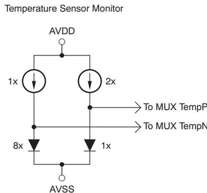
**Figure 19. Temperature Sensor Measurement in the Input**
