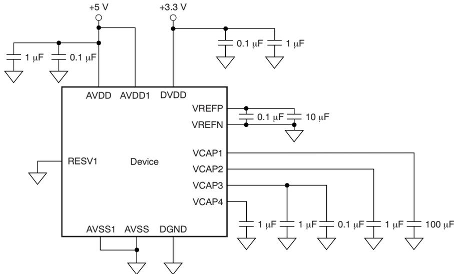
NOTE: Place the capacitors for supply, reference, and VCAP1 to VCAP4 as close to the package as possible.
