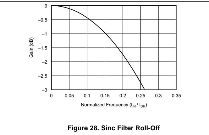
Figure 28. Sinc Filter Roll-Off
