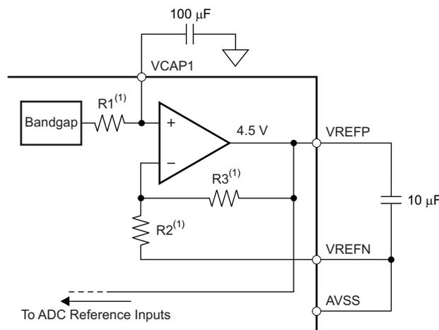
(1) For  $V_{REF} = 4.5\text{ V}$ :  $R1 = 9.8\text{ k}\Omega$ ,  $R2 = 13.4\text{ k}\Omega$ , and  $R3 = 36.85\text{ k}\Omega$ .
