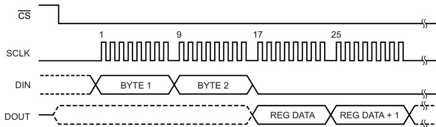
Figure 48. RREG Command Example: Read Two Registers Starting from Register 00h (ID Register)
