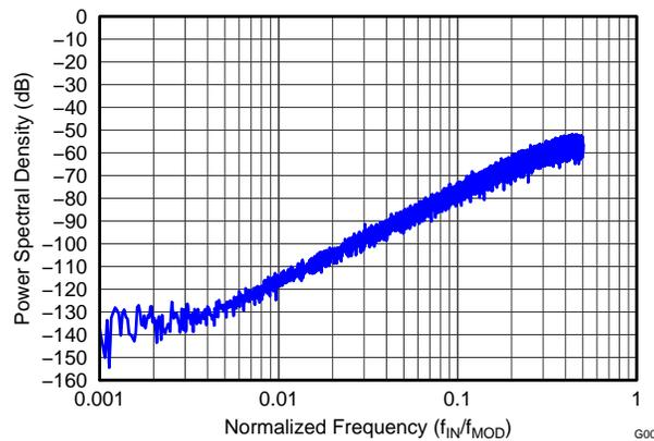
**Figure 24. Modulator Noise Spectrum Up To  $0.5 \times f_{MOD}$**
