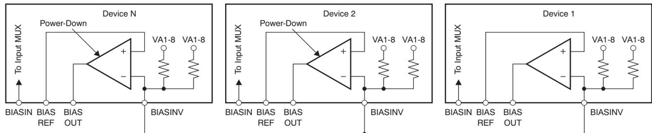
**Figure 39. BIAS Drive Connection for Multiple Devices**
