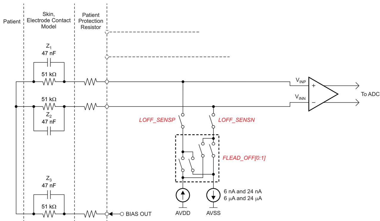
**Figure 35. Lead-Off Detection**
