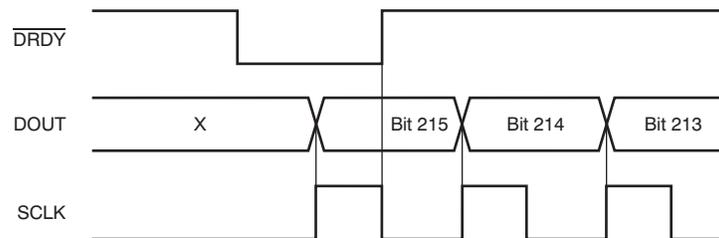
Figure 41.  $\overline{\text{DRDY}}$  with Data Retrieval ( $\overline{\text{CS}} = 0$ )
