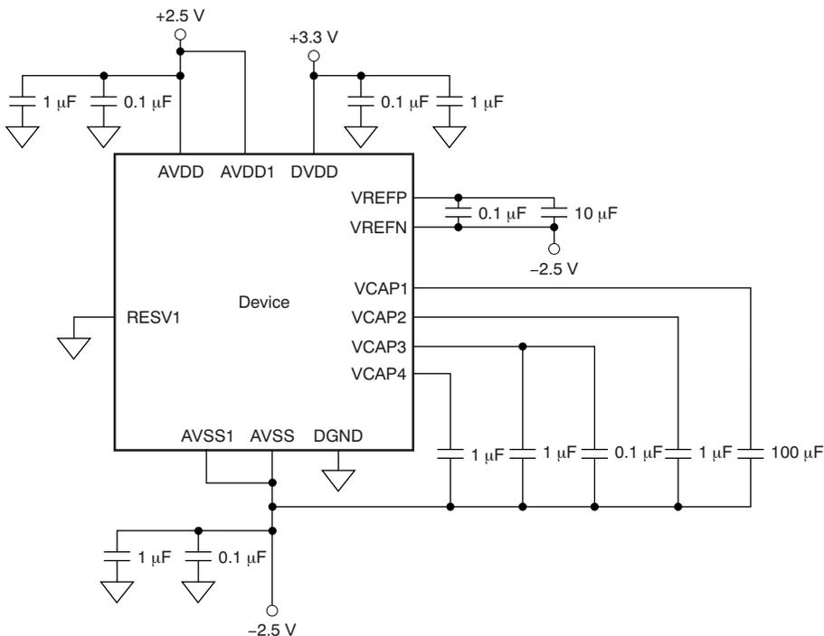
NOTE: Place the capacitors for supply, reference, and VCAP1 to VCAP4 as close to the package as possible.
